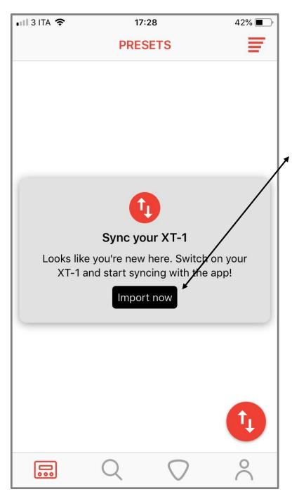
With your phone/tablet connected to the same Wi-Fi network of XT-1, or to the SIM1 Hotspot, import all the 30 presets of the pedal by clicking "import now".
