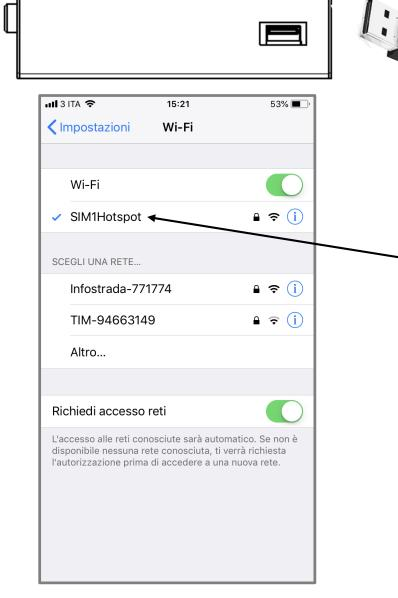
The app is now connected to "SIM1 Hotspot" of your device XT-1, through Wi-Fi System of your mobile/Tablet.
